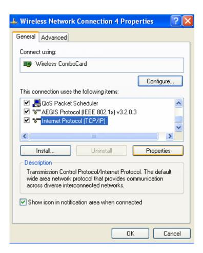
9. You can select either Obtain an IP address automatically or Use the following IP address setting. If your choice is the second one then entering the IP address, Subnet mask, Default gateway and DNS. After setting these parameters appropriately, click OK to make the changes work.
