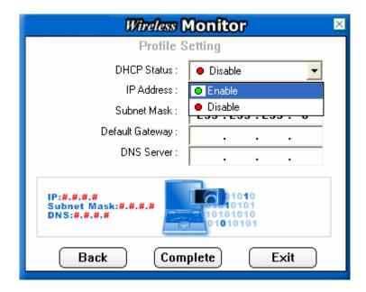
When the DHCP Status is Enable, the TCP/IP information will be assigned by a DHCP Server. Or otherwise please fill up with the correspondence data of the IP settings.
