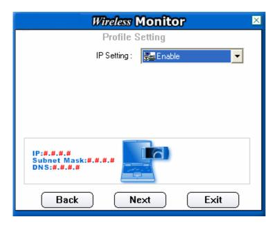
Please define if the current Profile IP setting will be assign by a DHCP Server or just assign by a fixed IP that is determinate by the Network Administrator.
